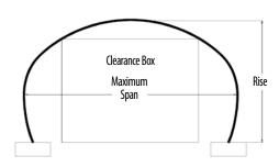
ALL DIMENSIONS ARE TO INSIDE CREST OF STEEL MINIMUM COVER IS FROM NEUTRAL AXIS OF STEEL CL Vehicle Minimum Cover
