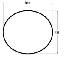
ALL DIMENSIONS ARE TO INSIDE CREST OF STEEL MINIMUM COVER IS FROM NEUTRAL AXIS OF STEEL CL Vehicle Minimum Cover CHBDC for Span > 3000 mm ASTM A796 (AISI) for Span < 3000 mm
