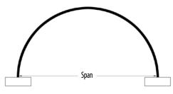
ALL DIMENSIONS ARE TO INSIDE CREST OF STEEL MINIMUM COVER IS FROM NEUTRAL AXIS OF STEEL CL Vehicle Minimum Cover CHBDC for Span > 3000 mm
